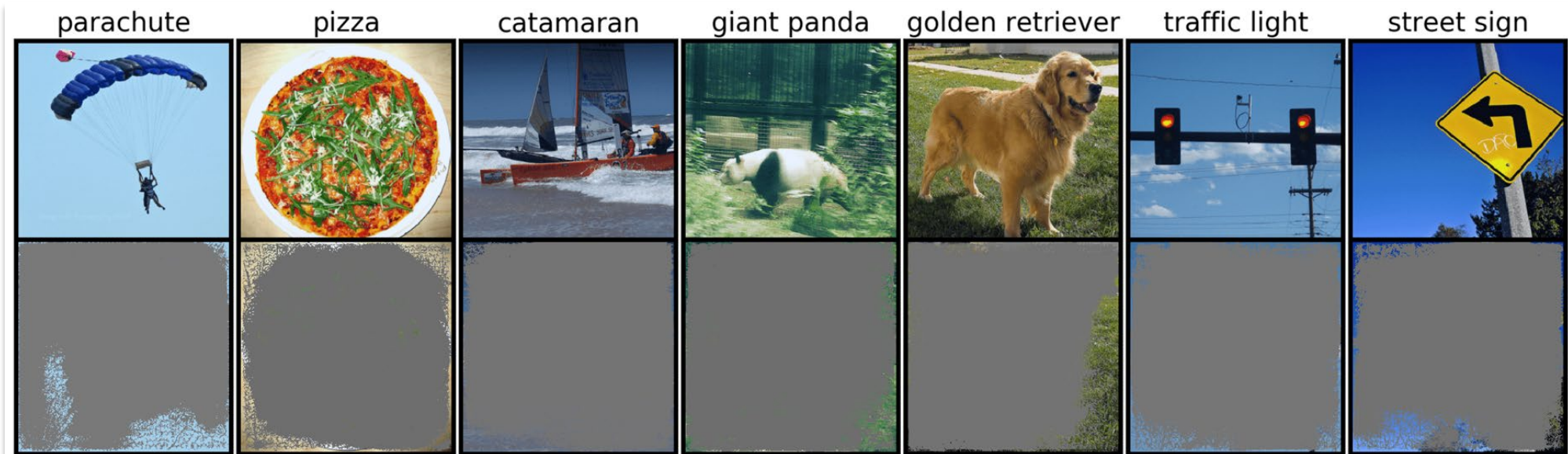
Figure 4: Sufficient input subsets (threshold 0.9) for example ImageNet validation images. The bottom row shows the corresponding images with all pixels outside of each SIS subset masked but are still classified by the Inception v3 model with \geq 90\% confidence.
